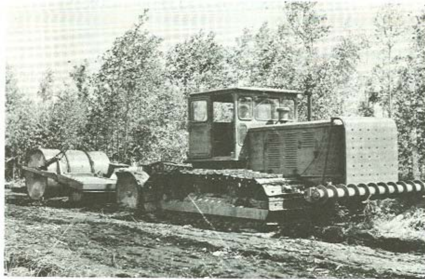
Figure 14.2 Machine MTP-42, which is used for continuous deep milling to 0.4 m depth and which can be used to create a fire barrier of moist peat
