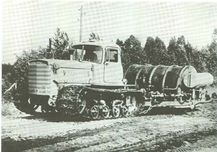
Figure 14.3 A fire suppression unit (AK-5P) which has a 5 m 3 capacity for liquid fire retardant
